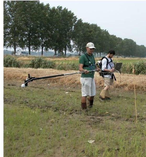
FieldSpec FR Pro, Analytical Spectral Device (ASD) (1nm, 4nm, 350-2500 nm)
